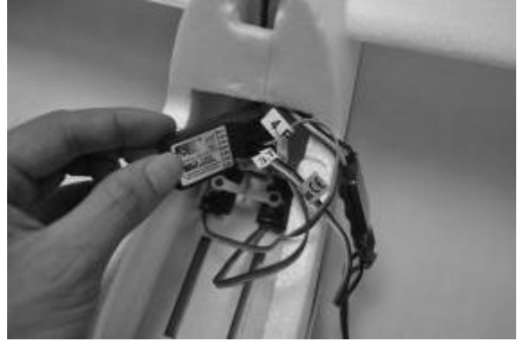
Fig.14- Connect the electronic speed controller and servos to the receiver .Refer to the radio instructions for the correct channel sockets and servo lead polarity .
