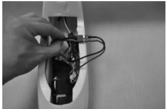
Fig.17- Photo shows battery leads connected to the electronic speed controller.
