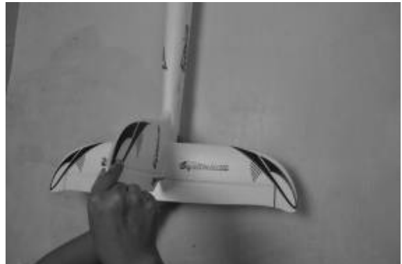
Fig.10- The photo shows Install the vertical stabilizers on the fuselage.
