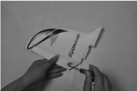
Fig.9- Fix the control rods with screws as shown in the photo.
