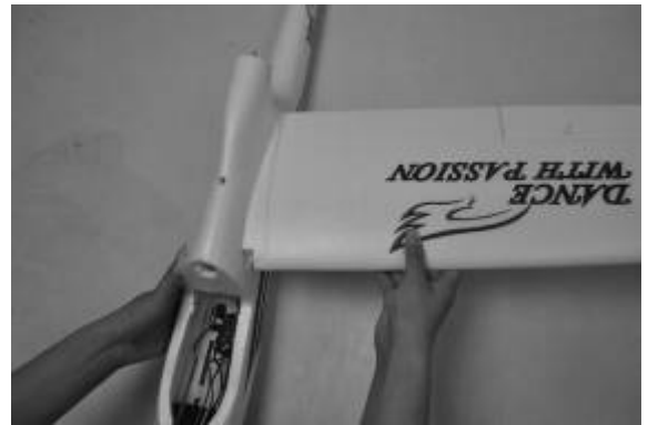
Fig.4- plug the main wing to the fuselage.
