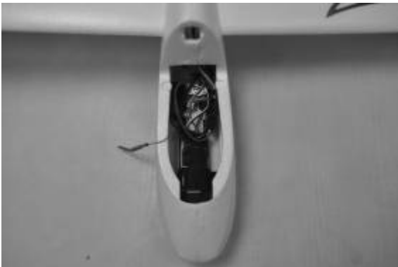
Fig.16- Photo shows the battery is installed in the fuselage
