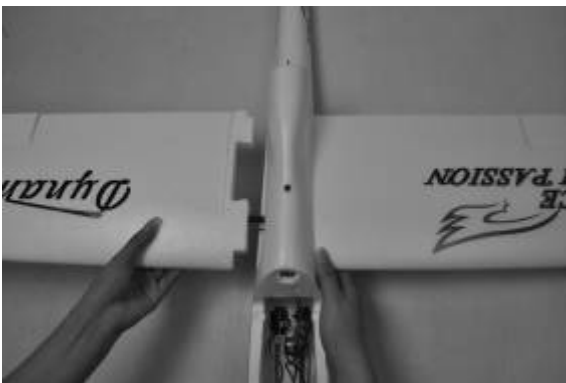
Fig.5-Pictures show the wing plug up to the side of each main wing panel.
