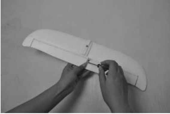
Fig.7- Fix the horizontal stabilizers control rods with screws as shown in the photo.
