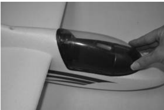
Fig.18 - Locate the canopy by the magnet, (One fuselage with two cockpit canopy)
