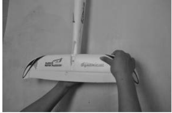
Fig.8- The photo shows Install the horizontal stabilizers on the fuselage.
