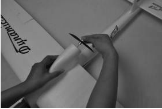
Fig.13- The photo shows the propeller is installed in the fuselage.
